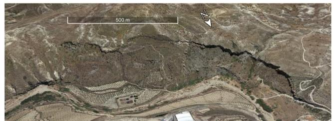
*Fig 2. Example of a post-capture, incision related landslide more than 1km across and more than one million cubic metres in size. Located above the capture point. Satellite image from Google Earth.*
