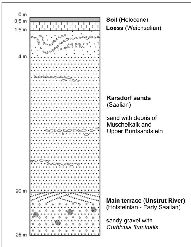
Fig. 8: Schematic section of the gravel-sand pit at Karsdorf (after MENG et al. 2006).
