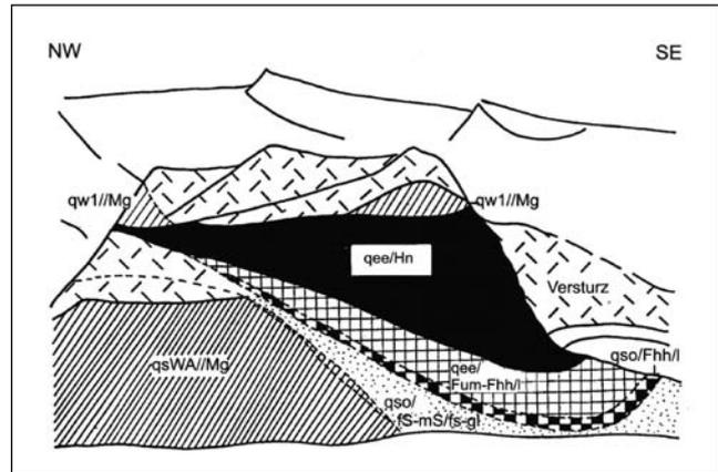
Fig. 4: Generalized geological cross section trough Eem outcrop Hinterste Mühle (at Profile 1) qw1//Mg = till, Brandenburg Stage, Weichselian-1; qee/Hn = limnic peat, Eemian; qee/Fum - Fhh/l = limnic silty mud and peat clay, Eemian; qso/Fhh/l = peat clay, Late Saalian; qso/fS - mS/gf-gl = glacio-fluviatile - glacio-limnic fine- and medium-grained sand, Late Saalian; qsWA//Mg = till, Warthe-Stage, Saalian-2 (STRAHL 2000)
