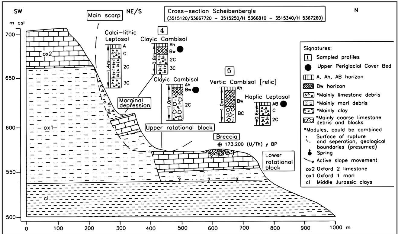
Fig. 5: Cross-section of the Scheibenberge landslide area (Stop 2) (TERHORST 2007).
