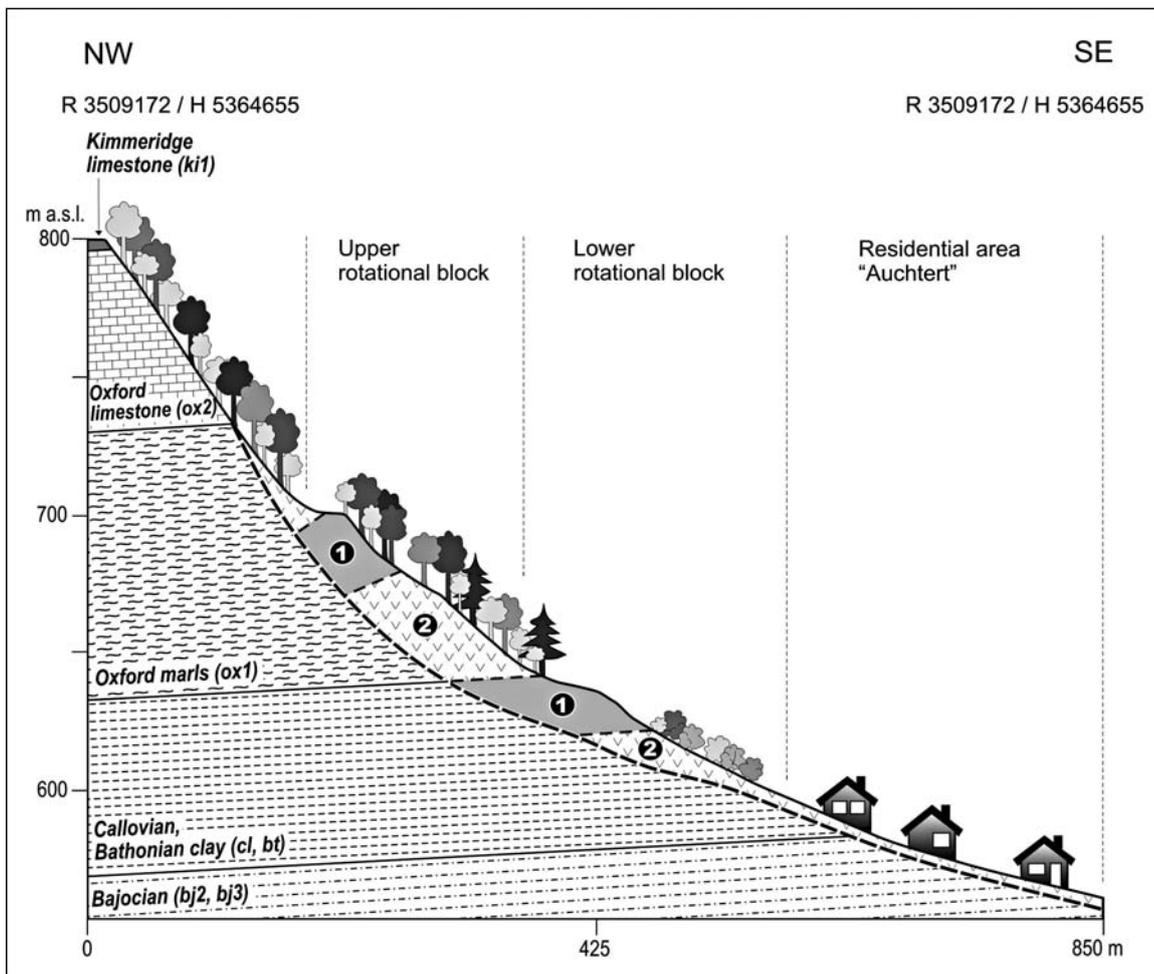
Fig. 10: Cross-section and slide masses of the Auchttert area at the Schönberger Kapf (Stop 4) (TERHORST & KREJA 2009).
