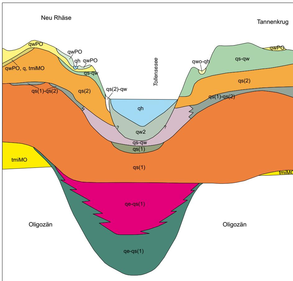
Fig. 3: Geological cross-section through Tollense-channel near Usadel (Source: LUNG M-V, Geological Survey)
