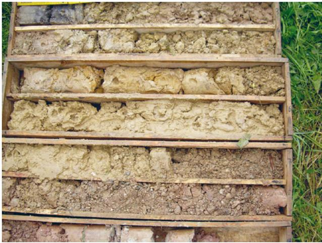
Fig. 14: Drill core near Eckershof (extract). 2–2.3 m black Lower or Middle Holocene buried soil overlain by colluvium; 2.3–6.6 m periglacial cover sediment; 6.6–ca. 8.3 m T2 gravel; >8.3 m Lower Triassic sandstone (sm).
