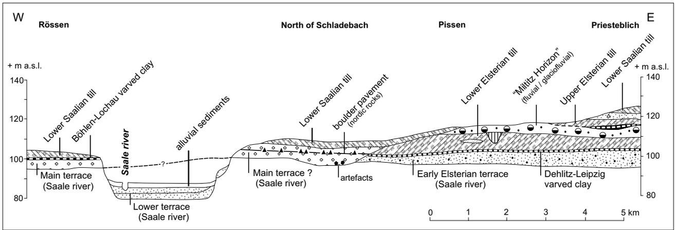
Fig. 3: Geological section across the area to the west and east of the Saale near Merseburg with exposed Wallendorf gravels (Main terrace ? in centre of section; after EISSMANN 1975).
