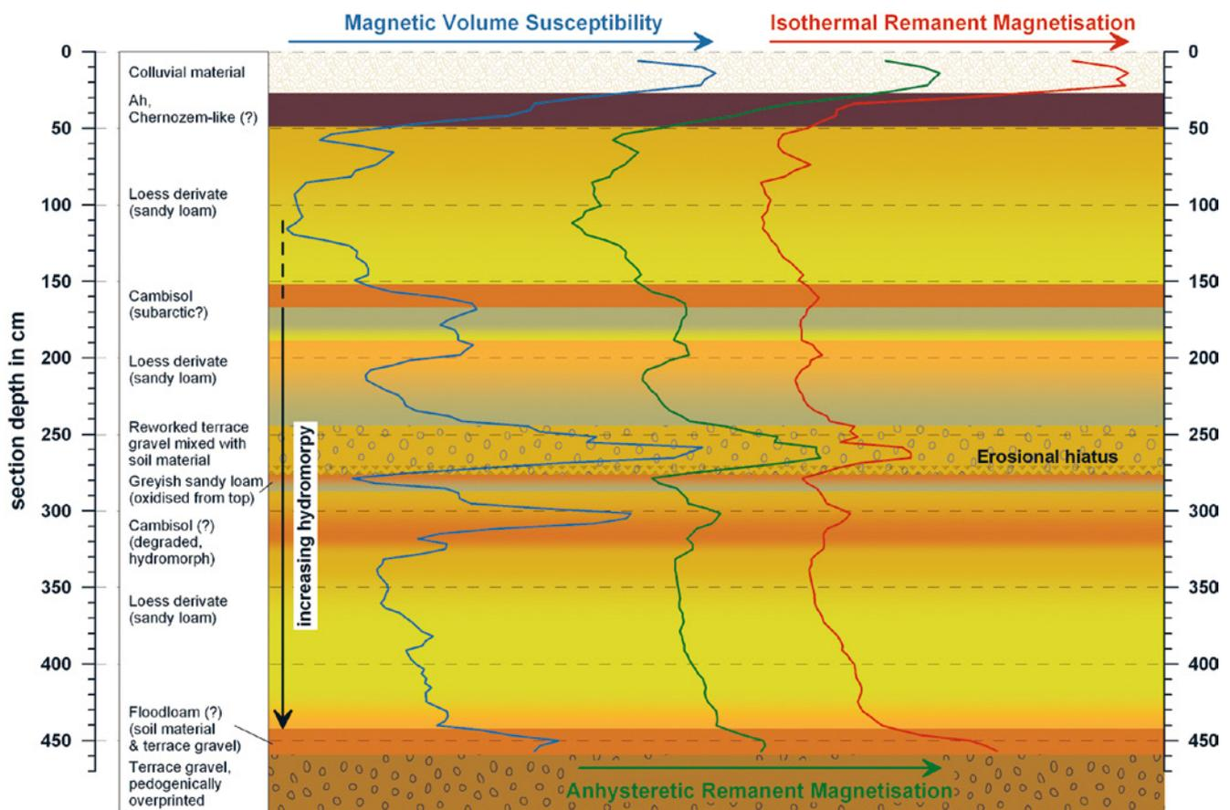
Fig. 10: Stratigraphic plot and selected results of rock magnetic measurements from the cover sediments of the T3 terrace at Bindlach. Magnetic Volume Susceptibility, Anhyseretic and Isothermal Remanence are displayed as function of stratigraphy. Elevated values are indicative for pedogenesis. Note the extreme values in the colluvium on top of the profile. Data treatment: outlier removal, detrending, normalising and smoothing.
